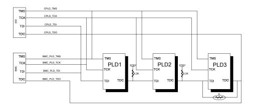
Figure 18. PLD Connections
